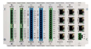
ensured that the required Ex-barriers are fitted in the control cabinet. They are not needed when using Ex-d sensors instead. In addition, the MFE7 can ensure the voltage supply to both current inputs and thus reduce the amount of wiring required. The HF inputs can be configured to work with pulse integrity checking according to ISO 6551 Level A.
