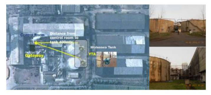
Modbus to Ethernet IP protocol converter was installed to establish the connection between the gateway and a host system, Allen Bradley PLC. These were located in the control room and antenna for the gateway was mounted outside using remote antenna cable to improve wireless quality.
